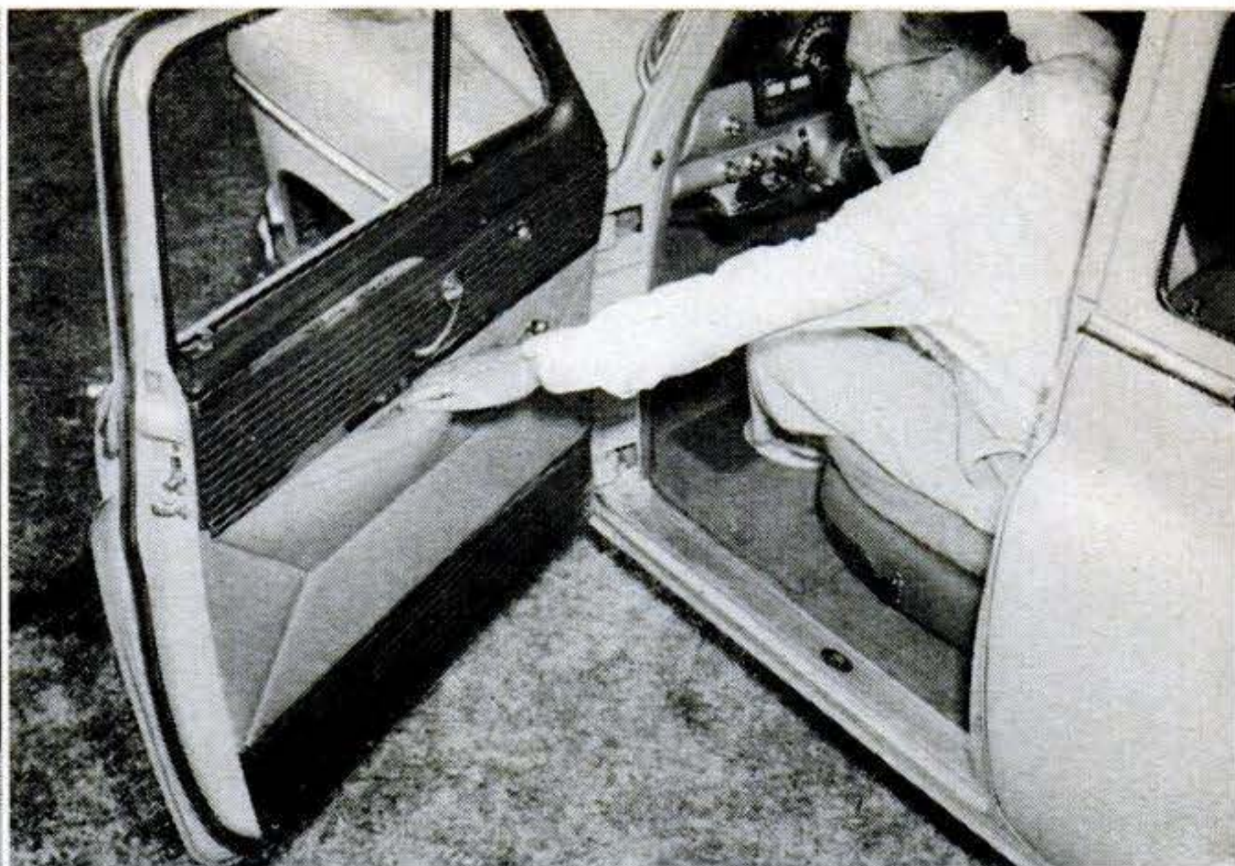
THE TRIM on the Oldsmobile has been fancied-up. There's a protective metal cup inside the door pull, and sure as shooting, some customers are going to use it for an ash tray.
